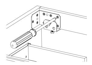
Screw the main body to the wall in order to bring more security to the installation.
