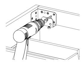
Drill an extra hole using the Decofix System as a guide to bring major strength to the union.
