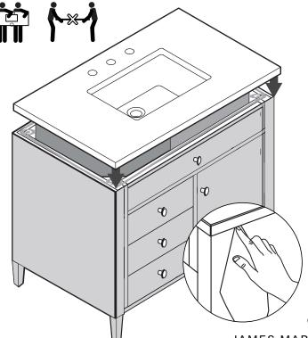
**10.** Once positioned, press firmly into place. Wipe away any excess sealant using a damp cloth.
