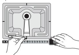
3. Carefully lift the sink and place it centered over the countertop cutout, bowl side up and with the overflow drain at the opposite end from the faucet holes. Align all marked center points along each side of the lip of the sink, with the marked center points along cut out in the countertop. Ensure the sink is centered over the opening and carefully trace around the perimeter of the sink with a marker.
