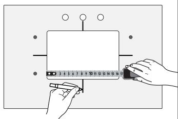
2. Carefully unpack the undermount sink and place on a soft surface, bowl side up. Using a tape measure, identify and mark center point on all sides of the bottom and profile of the lip of the sink.
