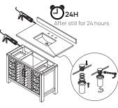
1.Install the water launcher
