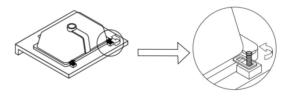
• Place and tighten the screws in the aligned holes.
