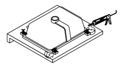
Apply caulk around the perimeter where the basin meets the countertop. Wait 24 hours for the caulk to dry fully.
