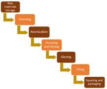
The required composition of raw materials, including also recycled wastes, is mixed and grinded in mills, either in a wet or a dry process.
