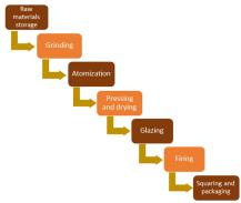
The required composition of raw materials, including also recycled wastes, is mixed and grinded in mills, either in a wet or a dry process.
