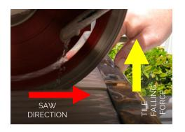
BECAUSE THE TILE WAS CANTALEVERED OFF THE RIGHT SIDE OF THE SAWS TABLE IT CREATED TENSION AT THE BLADE. THIS CAUSED A FAILURE AND THE END OF THE CUT.
